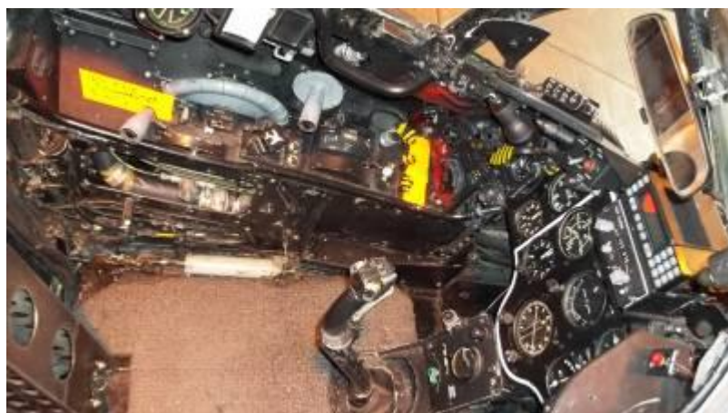
Right – innards of the Hawker Sea Hawk with Martin-Baker ejector seat removed.
